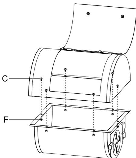
Please install and fix the ONE SIDE (Front) two holes to match the lid and fire bowl , then adjust the OTHER SIDE(Back) of the up and down hole position
