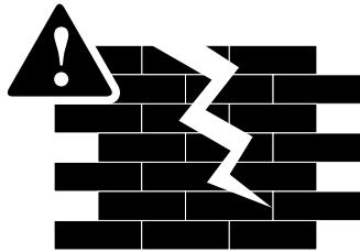
**Do not install on walls and ceilings made of: gypsum board, drywall, light processed blocks, silicate boards/bricks, a damp wall, weak or very old blocks or wooden panel! For installation on gypsum or light processed blocks please consult with an authorized installer or appropriate building specialist to install the product.**
