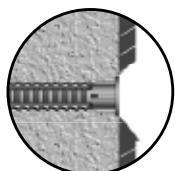
The anchor must be sunk up to 10 mm (3/8") into the plaster coating.
