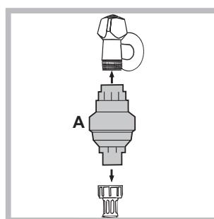
1. Connect the A device to a cold water tap using a 3/4 gas threaded attachment, then perform the connection by screwing the supply hose to the device.
